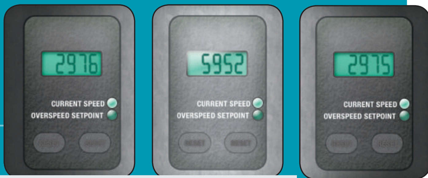
■ Figure 1. One of three speed indicators showing the double speed phenomenon (Middle).
